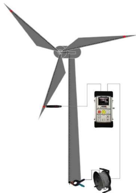
Lightning protection system testing with RMO-EH
